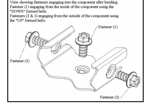
View showing fasteners being inserted during the assembly operation from different directions. Allowing for internal or external components to be fitted to the application.
