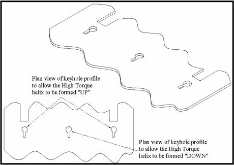
View showing pierce profile in panel during the manufacturing process, shape of keyhole aperture is relevant to the direction of the formed helix.
