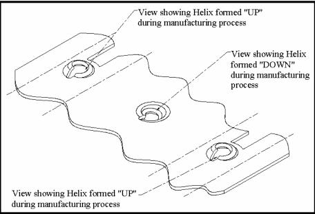
View showing helix formed in panel (UP and DOWN) during next manufacturing stage.
